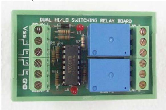
In this Version 2 PCB we have increased the board size to fit in a PCB carrier as shown in the photo. This DIN rail carrier is not supplied. It is just to show you. We have also added an LED across each relay to show when it is activated.
